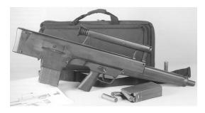
The FC CAWS is a select-fire, smoothbore weapon, designed to fire special, high-pressure shotshells, loaded with tungsten buckshot or flechettes. FC CAWS utilized a patented recoil-operated action with a moving barrel and an additional, self-regulated gas assist system (used to help unlock breechblock from the barrel if low-power ammo is used). The main goal of this system was to decrease felt recoil down to a suitable level.
