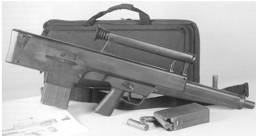
The FC CAWS is a select-fire, smoothbore weapon, designed to fire special, high-pressure shotshells, loaded with tungsten buckshot or flechettes. FC CAWS utilized a patented recoil-operated action with a moving barrel and an additional, self-regulated gas assist system (used to help unlock breechblock from the barrel if low-power ammo is used). The main goal of this system was to decrease felt recoil down to a suitable level.
